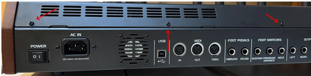
5. You can now lift and flip the top cover to the back. The top panel is kind of hinged to make this process easier. It stays open on its own.
