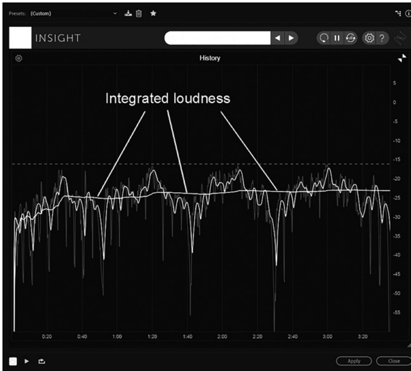
Figure 19.2 Example of a level recording in the form of Loudness Level.
