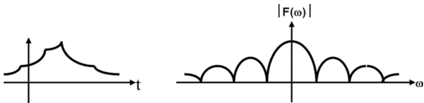
Figure 26.3 Left: Nonperiodic signal. Right: Continuous frequency spectrum for a nonperiodic signal.
