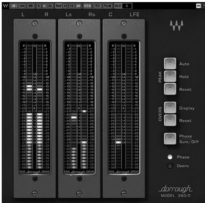
Figure 14.1 The Dorrough Loudness Meters provides readings of the peak and the average program level simultaneously.
