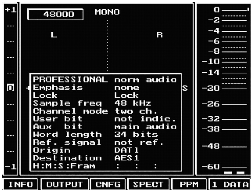
Figure 23.3 Significant information gathered from channel status and made available on the screen of the instrument. Among other things, you can see that this concerns professional/two-channel audio/48 kHz/24 bit/without emphasis/no time code.
