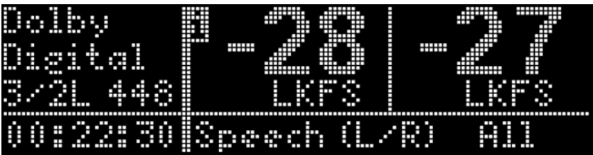
Figure 14.2 An example of the display readout on the Dolby® LM100.
