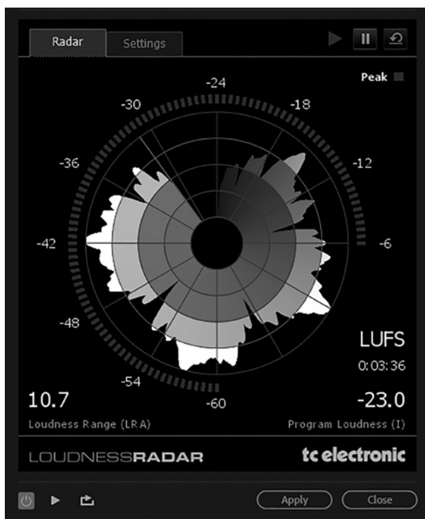
Figure 14.7 The characteristic radar display on LM2n from TC Electronic. The speed of the radar can be set.
