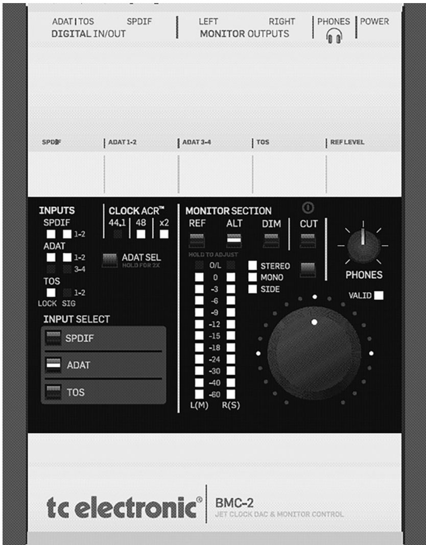
Figure 25.14 An example of a combined D/A converter, meter, and monitor control unit for loudspeakers and headphones. Digital inputs are S/PDIF, AES3, TOS, and ADAT (including the ability to confirm whether those inputs are synchronous or not). (TC Electronic, BMC-2).
