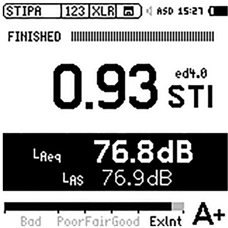
Figure 28.8 STI-PA readout from a handheld device (NTI AL1 Acoustilyzer). The display shows that the measurement is finished and that the value is 0.89, which corresponds to “Excellent” or A+.
