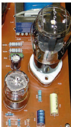
All components on one side of the PCB (Top side)
