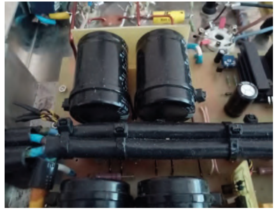
Auxiliary PCB - horizontal mounting of capacitors
