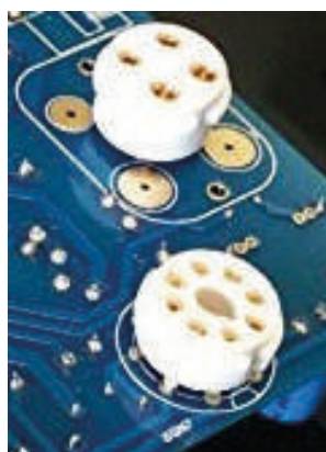
Tubes sockets on one side of the PCB (Cu side)
